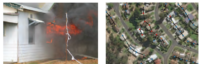
Figure 4: Left, experimental house fire and radiometers. Right, consequential fire probability.
