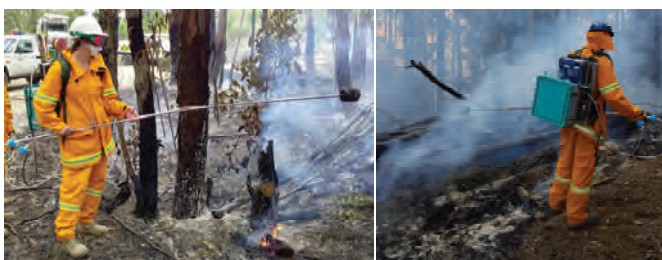
Figure 1: Examples of sampling from smouldering combustion using portable backpack smoke collectors. Filter holders can be seen in blue. Backpack contains DustTrak-II, Q-Trak, two pumps, gas meter, batteries and a Tedlar bag house within the green box.
