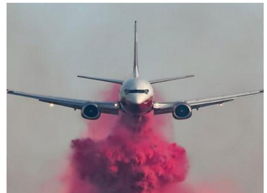
The LAT will fly to anywhere in Australia within hours and drop 15,000 litres of retardant or water on a fire.
