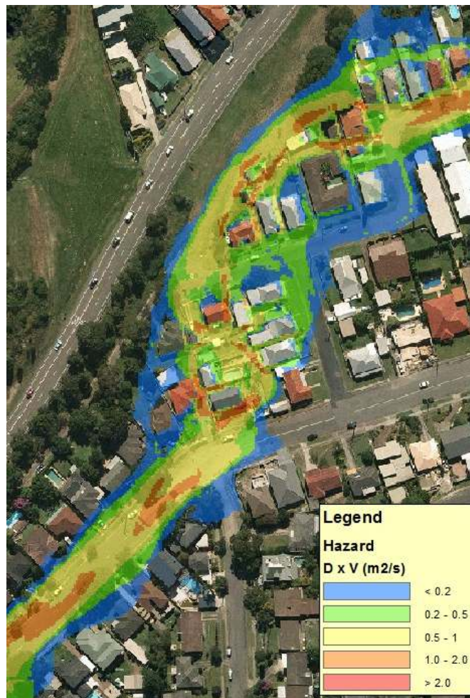
Figure 4: Example of peak modelled D x V (Source: Smith and Wasko, 2012)
