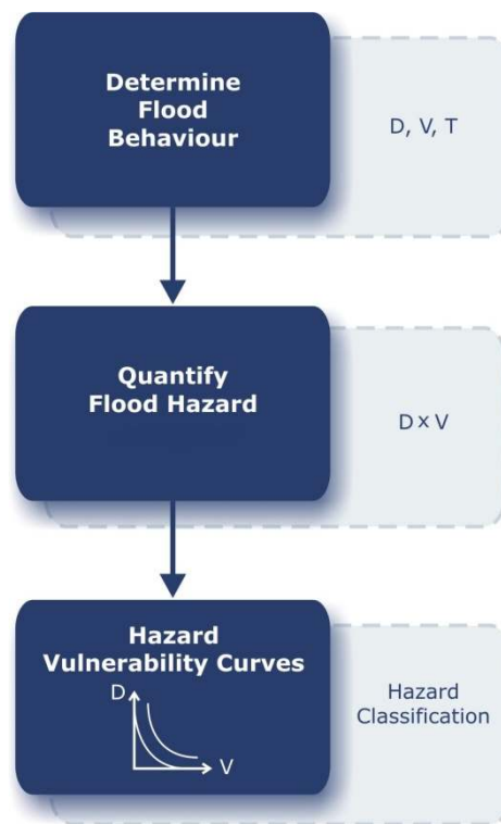
Figure 2: Process for quantifying flood hazard
