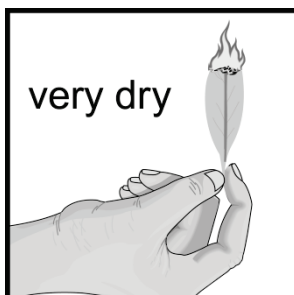
Figure 19: Estimating FMC from burning-leaf test (using a dry eucalypt leaf) (Source: DELWP, Vic.)
