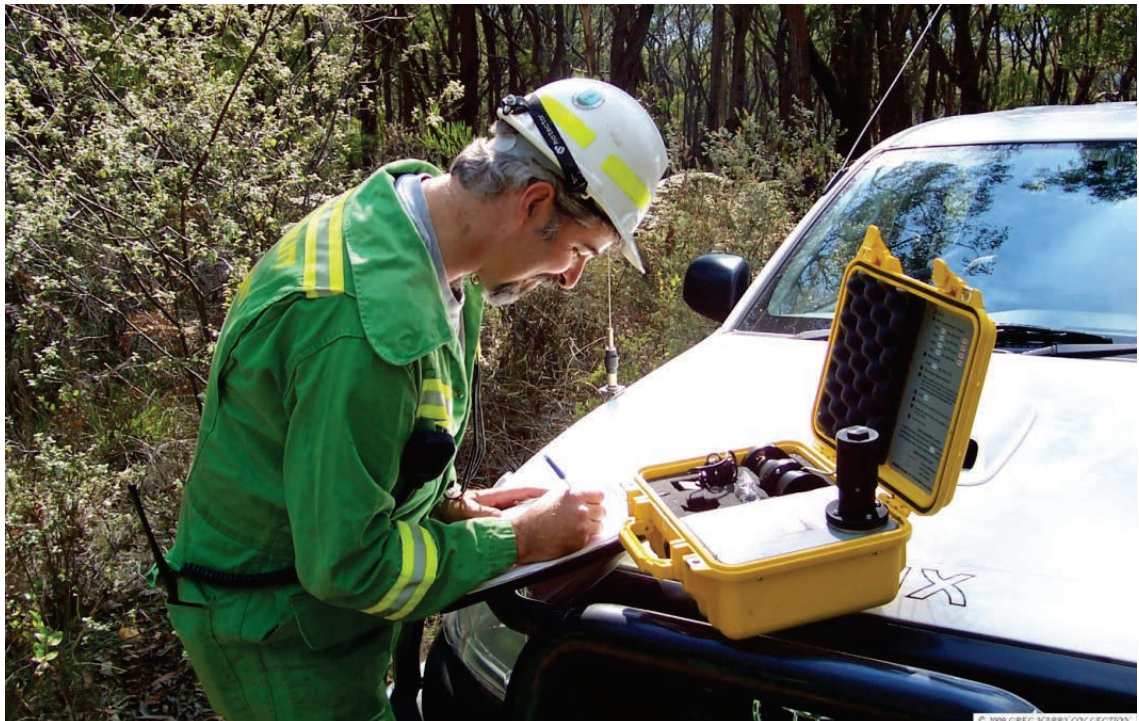
Figure 42: Using an electronic fuel moisture meter (Source: DELWP, Vic.)
