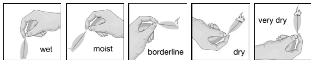
Figure 49: The burning-leaf test
