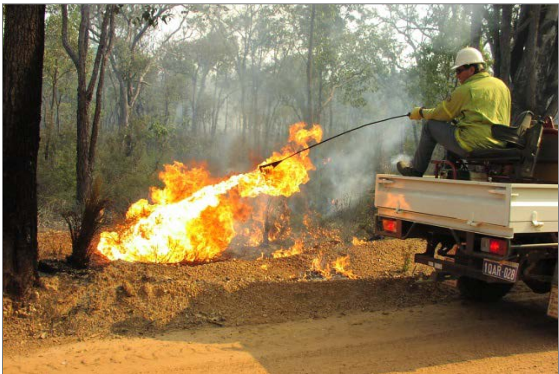
Figure 31: Vehicle-mounted flame thrower (image courtesy of DPAW, WA)
