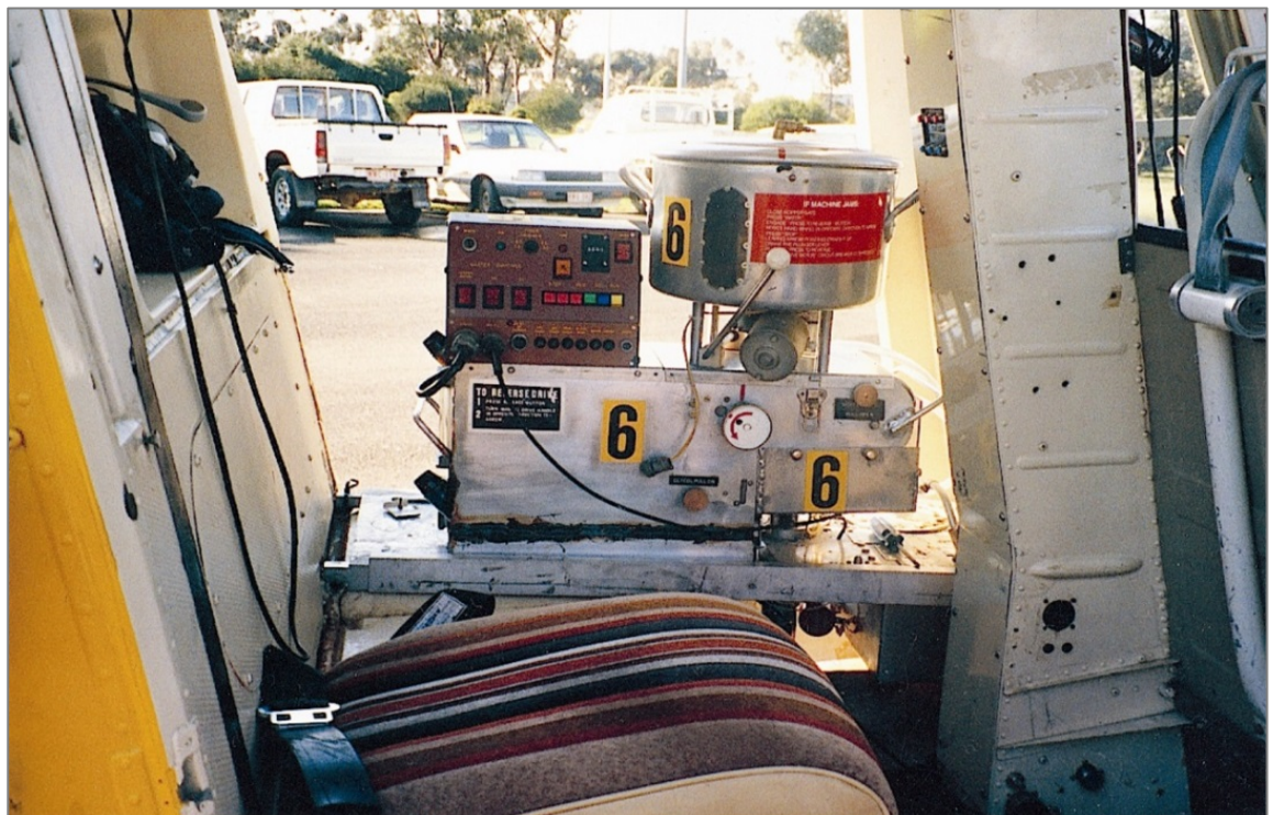
Figure 32: Aerial incendiary machine in a light helicopter
