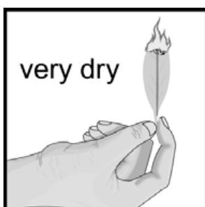
Figure 22: Estimating FMC from burning-leaf test (using a dry eucalypt leaf) (Source: DELWP, Vic.)
