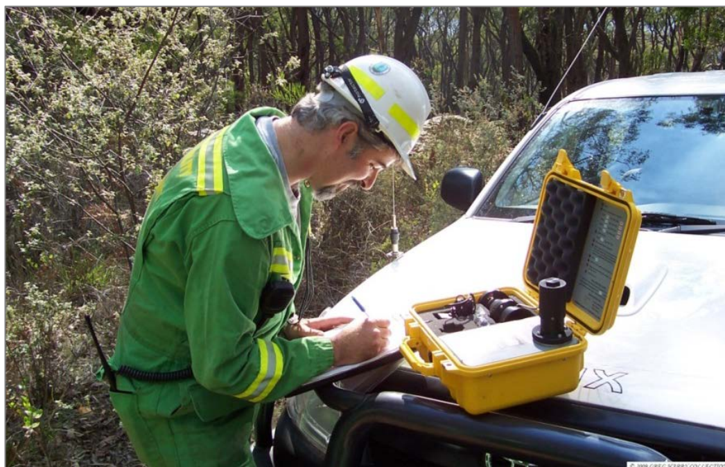
Figure 53: Using an electronic fuel moisture meter (Source: Department of Environment, Land, Water and Planning Vic.)
