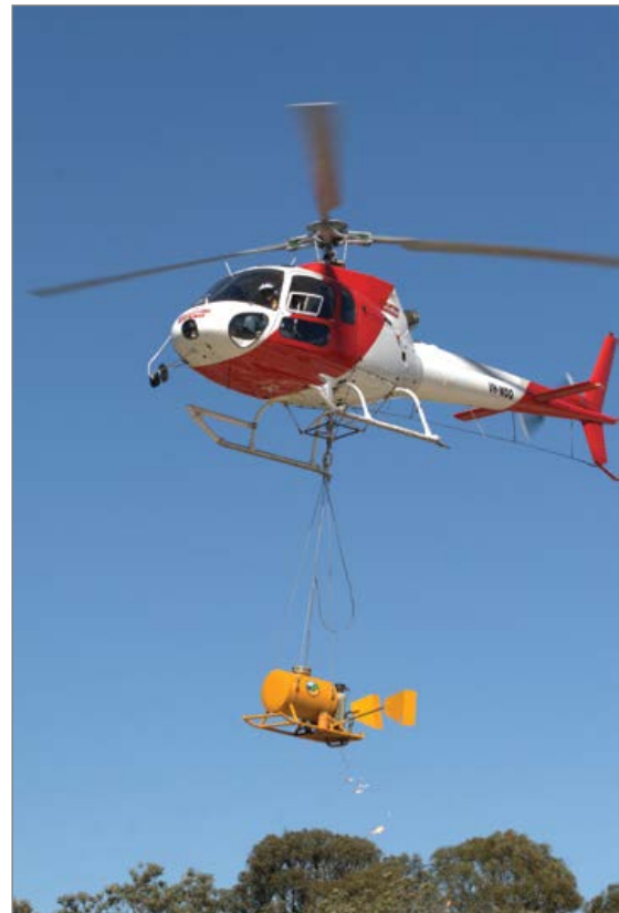
Figure 30: Aerial driptorch slung beneath a light helicopter
