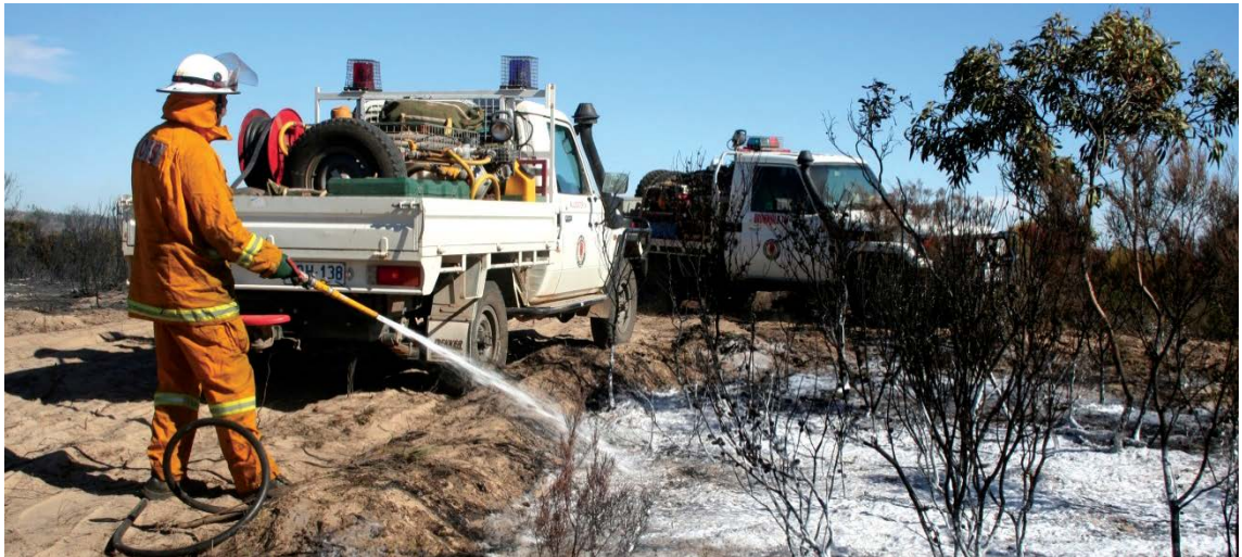
Figure 42: Foam applied to ensure uniform coverage during mop-up (Photo courtesy of Bushfire CRC)
