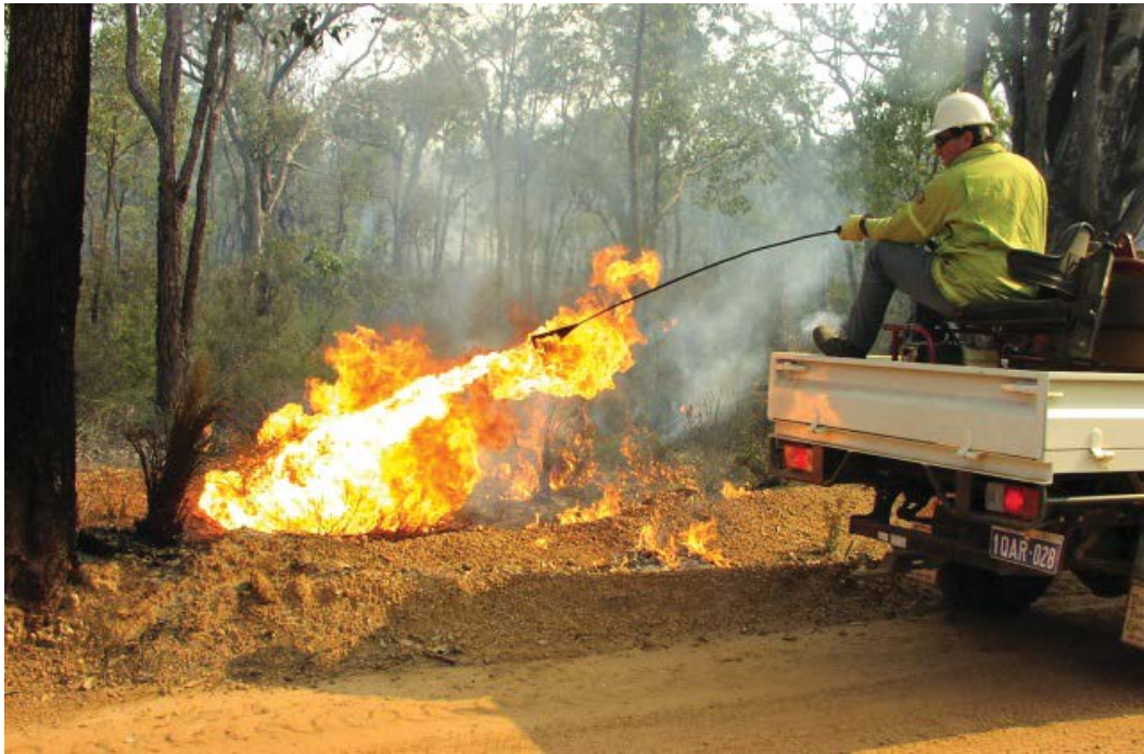
Figure 22: Vehicle mounted flamethrower (Source: DPAW, WA)
