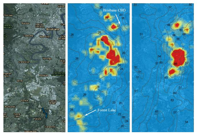
Figure 5: Region of RDA analysis (left), wind damage point density (centre) and hail damage point density (right) based on RDA analysis region. Wind speed (m/s) contours (centre) and reflectivity (dBZ) contours (right) based on radar data analysis.
